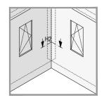
WL132C.1-H2.1 Horizontal section - interior corner without expansion joint
