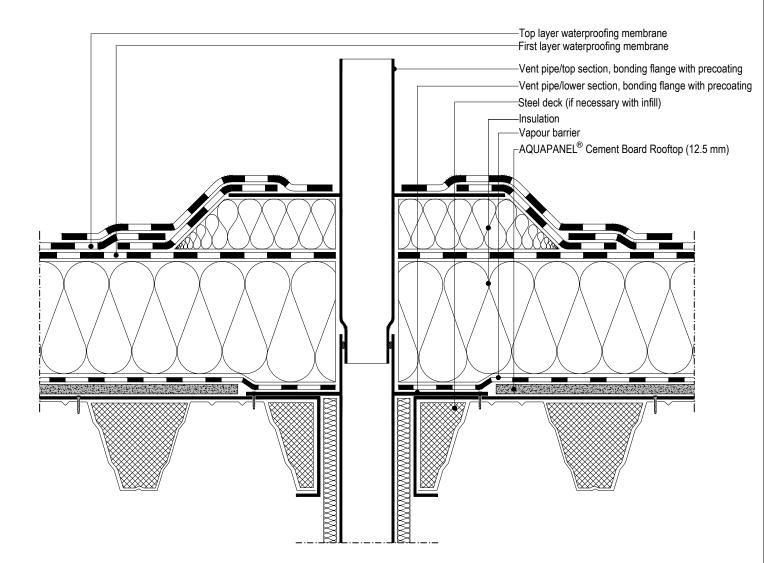
The drawings illustrating the general concept of how the system works and interfaces with other construction components. The drawings do not substitute an execution design.
